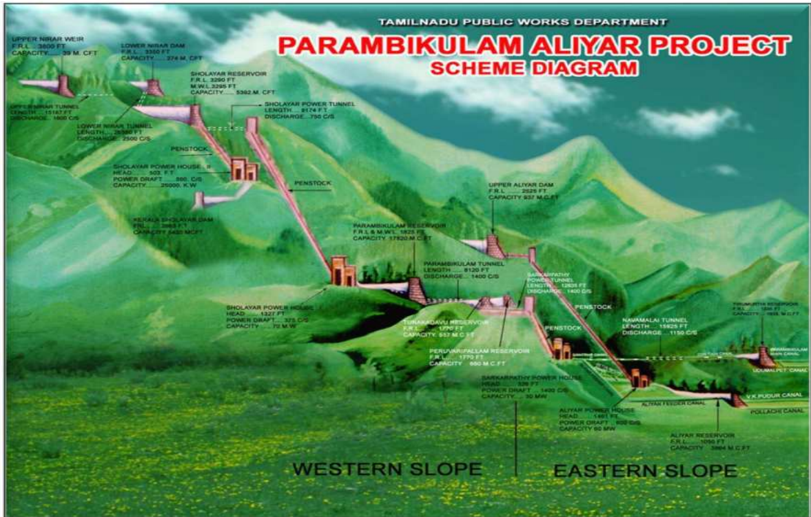
FIG. 1: PAP SCHEMATIC LAYOUT OF RESERVOIRS
